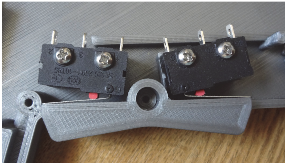
FIGURE 7 – Switches and trigger; the metal lever just touches the trigger
