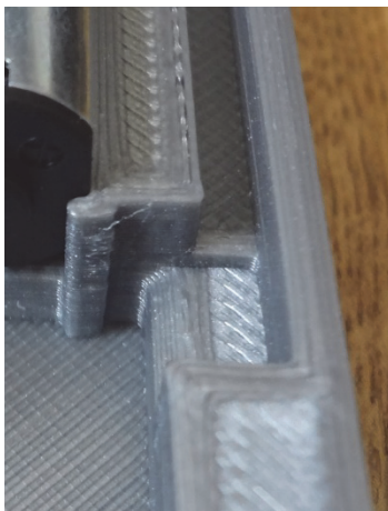
FIGURE 13 – Pillar keeping the MT3608 module in place
