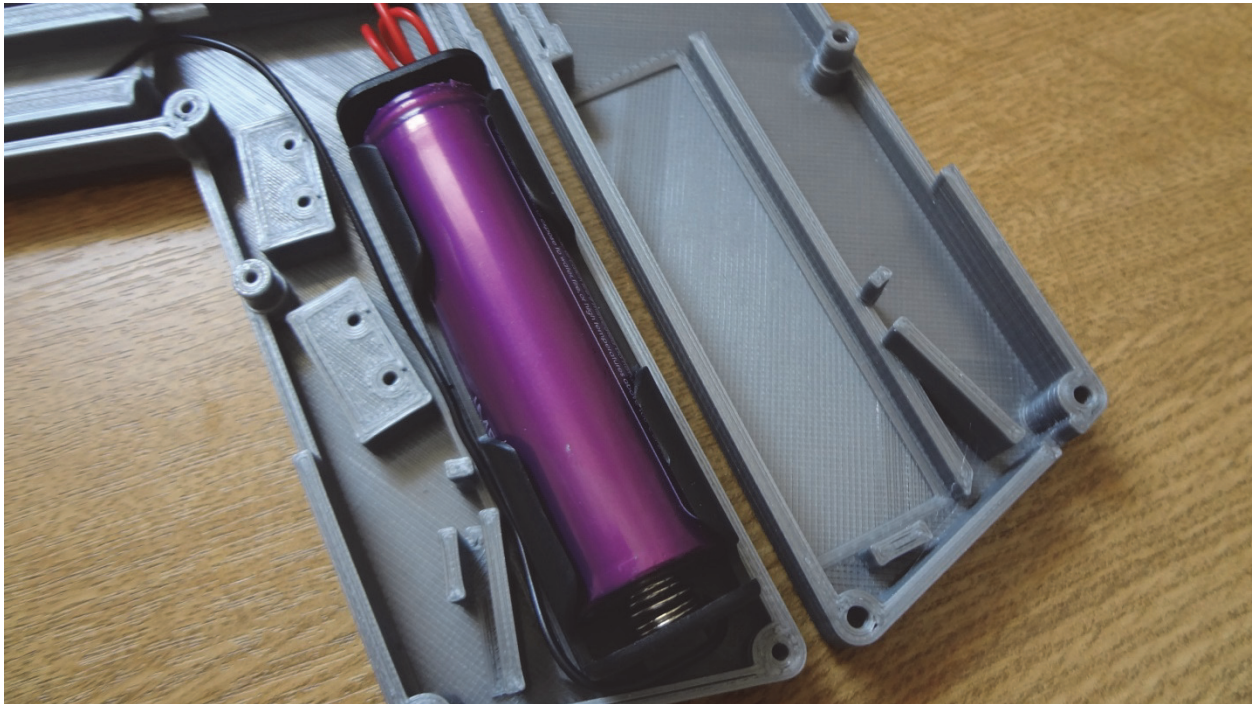
FIGURE 12 – Right and left covers; the wide groove for the battery is seen in the left cover (right side of the image)
