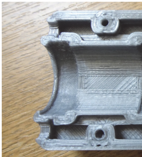
FIGURE 14 – Holes for the LEDs, at each side of the front bearing groove
